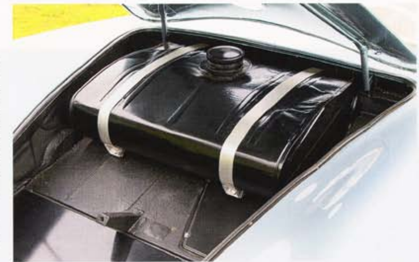
Left: Through-hood fuel filler feeds a tank that dominates the luggage bay. Below: The Sauter roadster (#12) at Monaco in 1952, racing thru the chicane.
